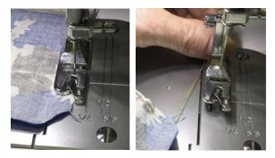
The foot has a corkscrew like apparatus in the front that double turns the fabric just before it reaches the needle. Most narrow hemmer feet are designed to be used in the center needle position. The fabric feeds through the foot with the raw edge of the fabric fitting in the groove just to the left of the corkscrew and the fold of
