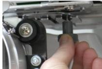
Carefully slide the cap frame driver onto the machine. The square opening fits into the freearm of the machine. Don't hit the needles with the top of the cap frame driver. (**Don't hit the needles with the cap frame driver!**) Align the loosened large thumbscrews on the bottom of the cap frame driver and the top holes onto the pegs. The small thumbscrews will fit into the v-shaped slots to the right of the holes on the top of the cap frame driver.
