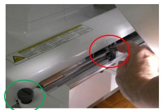
The Frame Holder is the part that attaches to the machine and the hoop (frame) slides into the frame holder. Different hoops use different frame holders. The Array comes with two frame holders, the white "A" frame holder and the grey "B" frame holder. The four hoops that come with the machine use the "A" frame holder. The "B" frame holder is for some of the optional hoops such as
