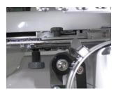
Finger-tighten the thumbscrews to secure the cap frame driver. The cap frame driver should just clear the free-arm of the machine. To adjust the height of the cap frame driver, follow the explicit instructions in the user manual.
