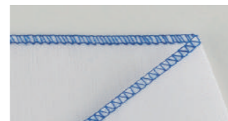
3-Thread Narrow Overlock The fabric edge is rolled, then sewn with very narrow overlocking.
