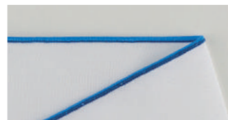
3-Thread Rolled Hem The fabric edge is rolled, then covered with thread.
