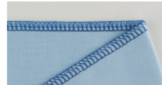
4-Thread Overlock Uses 2 needles and 4 threads to securely sew together knitted fabrics.
