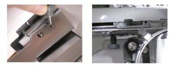
Finger-tighten the thumbscrews to secure the cap frame driver. The cap frame driver should just clear the free-arm of the machine. To adjust the height of the cap frame driver, follow the explicit instructions in the user manual.
