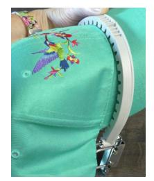
Sometimes the seam will not completely fit into the little teeth, so fit the center area as best as you can. Pull the sweat guard (the little flap of fabric in the inside of the cap) away from the cap and underneath the pins on either side of the upper frame. Drop the upper hoop fitted with the cap straight down onto the mounting jig and insert the bottom of the u-shaped piece into the openings on the frame. With your thumb on the pin on the
