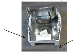
the upper frame by turning the lock knob to the unlocked position. Pull the upper u-shaped part up and off of the hoop. Using the metal extensions on either side of the hoop (they look like ears) push the hoop onto the mounting jig. Look on the top of the mounting jig to see that the center notch fits onto the center mark on the mounting jig. The frame will click into place with minimum pressure.
