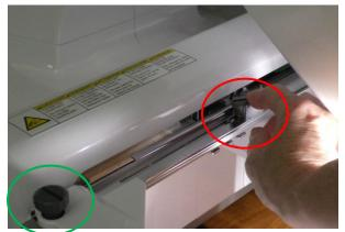
The "Cap Frame Driver" is the part that attaches to the machine. To install the new part, turn off the machine. Seriously, you don't want to accidentally make the machine move as that would not be good for the machine or for your fingers. Remove whatever frame holder currently attached to the arm of the machine. There are two small-ish thumbscrews on the top of the frame holder (red
