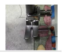
Set up sewing machine for straight stitch and stitch length of 2.5mm. Stitch just inside and
