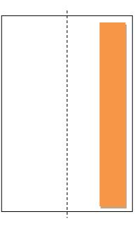
Select a quilting design and thread the machine with a thin thread through the needle. The bobbin thread will not show in the finished quilt, so use either embroidery bobbin thread or piecing thread in light color. Hoop the quilt with the narrow edge of batting on the right side of the hoop.
