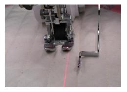
The key to beautiful grid quilting is consistent direction and width of the quilting lines. Use the LED guide light and needle position to sew straight and even lines. A quide bar attachment is available for the Digital Dual Feed. Mark the first line with a removable marker and use the light or quilt guide attachment to sew the rest of the lines without marking.
