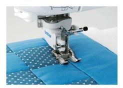
This foot attaches directly to the machine and is not a snap on foot. Secure the foot well when attaching the foot so it doesn't work loose while stitching. On the right side of the foot the leaver has a plastic "C" shape on it's end. This cups over the needle clamp screw and creates the action of the foot while stitching. Place this leaver in position before positioning the foot onto the ankle screw.
