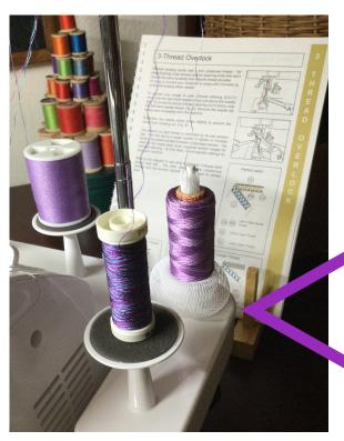
Because the thread for the upper looper was very slippery and wanted to fall off the spool, I used one of the thread nets that come with the machine as shown in the photo. Insert the thread net in the bottom of the thread and puddle the net around the bottom of the spool.
