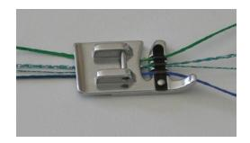
Adjustable couching feet can accommodate a variety of size strands. The opening has a sliding support that can be adjusted to keep the fiber centered. Load the fiber and adjust the size of the guide before attaching the foot onto the machine.
