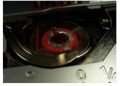
movement of the thread through the system. Bobbin tension is a resistance system created with the bobbin tension spring. Thread travels through the spring when threading and placing the bobbin in the machine. In the Stellaire, the quick set bobbin system automatically places the bobbin thread in the correct location. You can tell a correctly threaded bobbin when the thread is visible in diagonal line from the left to right across the top of the bobbin *after the first stitch*. See the photo.
