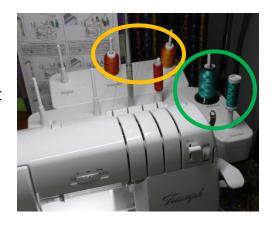
your fingers or along the edge of a table to set the stitch and even it out. Don't use very thick or bulky threads with these stitches. As shown in the photo, place two 40 wt. embroidery threads (orange and teal) on the additional spool pins and thread through the loopers as one thread. The Baby Lock Exclusive Wave stitch is available as a narrow rolled hem.
